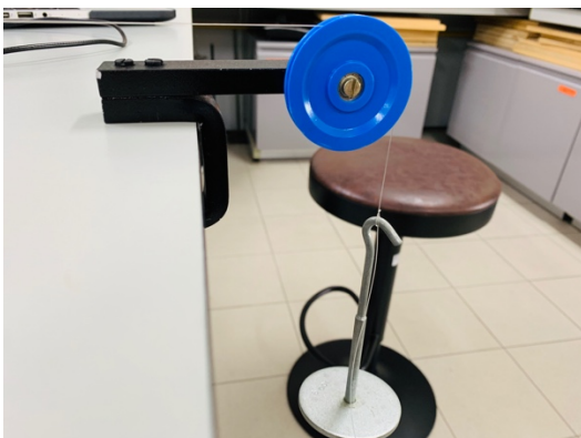
Figure 3 A close-up shot on the pulley clamp and the masses
