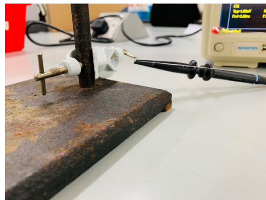
Figure 4 A close-up shot on the probe and the string
